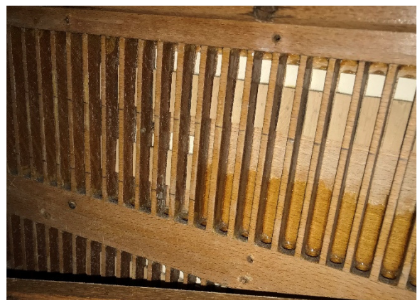
Coupler clack valves & channels
