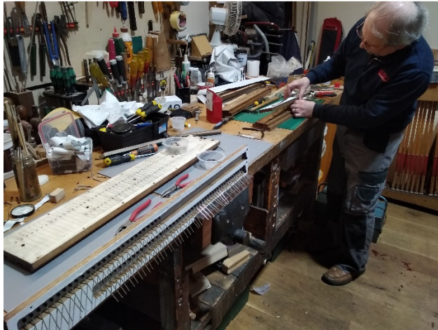
Restoring coupler action - 1
