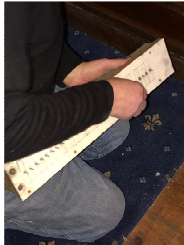
Removing coupler action
